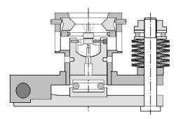
Figure 1: Side view of the shear cell with garnet anvils.
