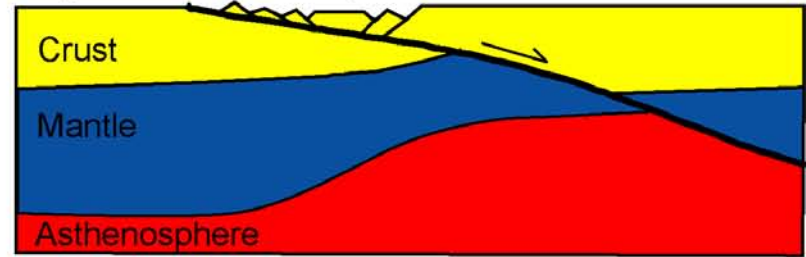
Asymmetric 'Simple Shear' Rift Mode
