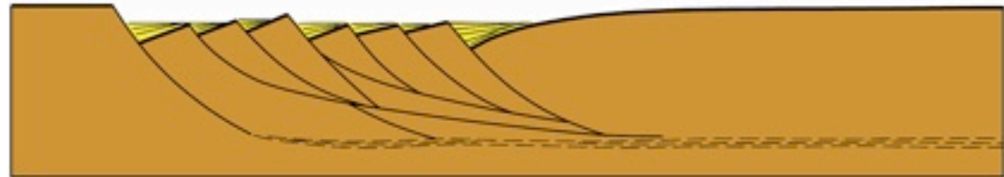
b Low-angle normal faults "fire" from delaminating layer
