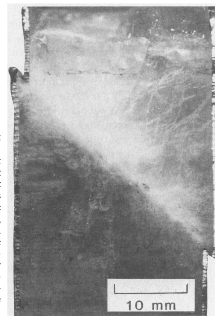
Fig. 5. Sample that faulted at high pressure (run 263, T = 77 \text{ K} and P_c = 100 \text{ MPa} ) cut perpendicular to the fault plane. Fault is inclined at about 45^\circ to \sigma_1 . Cohesion is maintained and the shear zone contains fine-grain ice II, which scatters light more than the host ice I, and therefore appears bright. Fractures radiating from the fault probably occurred when the jacket ruptured and the inert fluid confining medium entered the sample under load.
