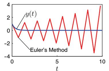
Figure 8.1 Euler's method is unstable for  $\tau > 2/\gamma$ . ( $\tau = 2.1/\gamma$  in this case.)
